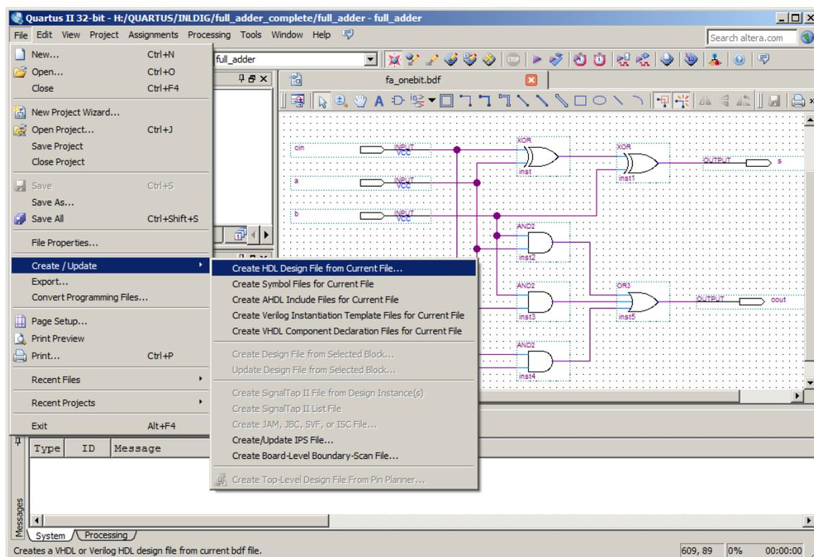
Figure 1: Converting a Block Design File to an HDL File.
